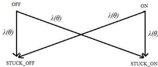
Fig. 8. States and transitions of the components.
