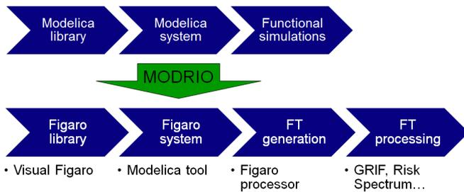
Fig. 2. The design and dependability analyses workflows at EDF.
