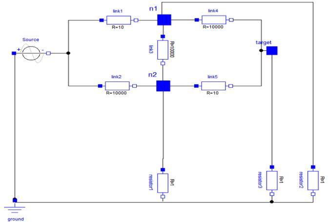
Fig. 5. Analog model of a telecom network: electrical circuit.
