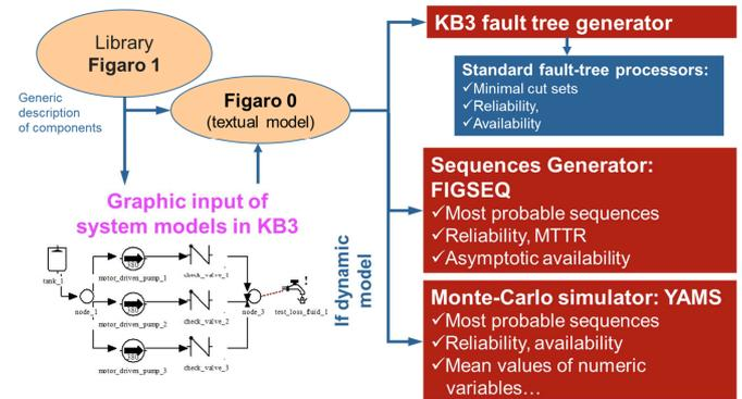
Fig. 1. The Figaro workbench overall architecture.
