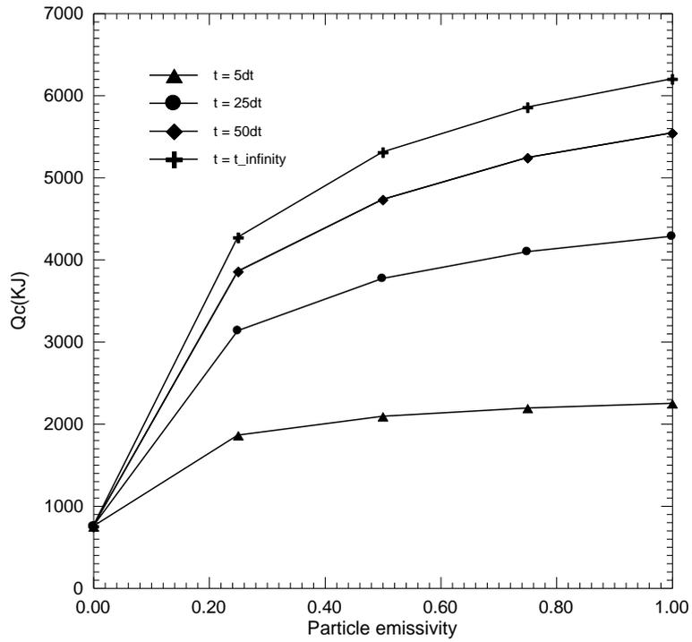
**Figure 2.** Amount of heat transferred to the fluid as a function of  $\epsilon$  for various time values.
