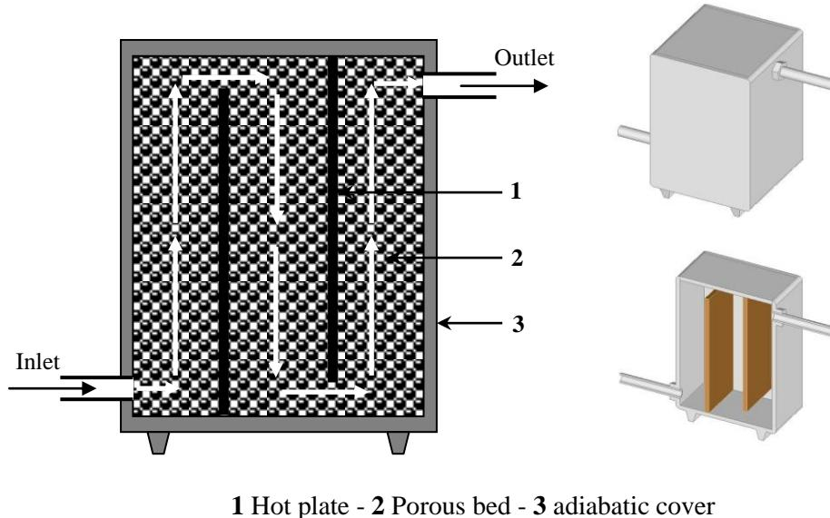
**Figure 3.** A skeleton of a heat exchanger including a porous bed formed by high emissive spherical particles
