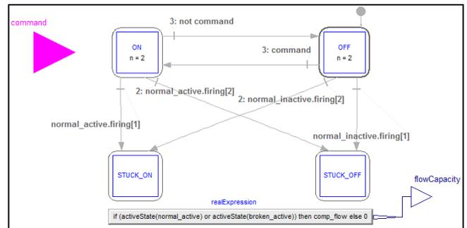
Fig. 10. Continuous-time state-machine model for the two pumps and the valve.
