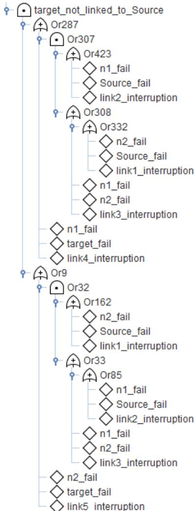
Fig. 6. Fault tree generated from the telecom network.
