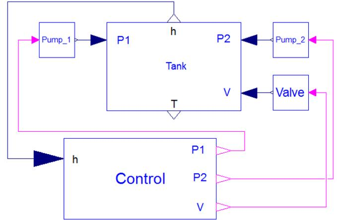
Fig. 9. Structure of the Modelica model.
