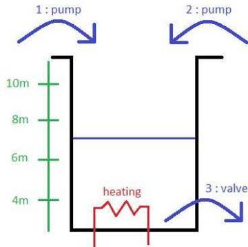
Fig. 7. The "heated tank" system.
