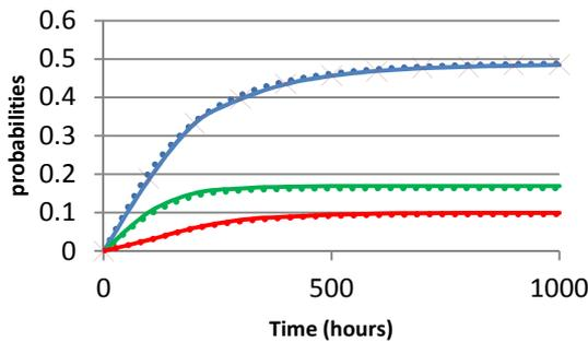
Fig. 11. Cumulated probabilities of failures. Comparison between our results (105 histories) and PDMP from Zhang et al. (2009) (107 histories, dotted). Blue: overflow; Green: boiling; Red: drought.
